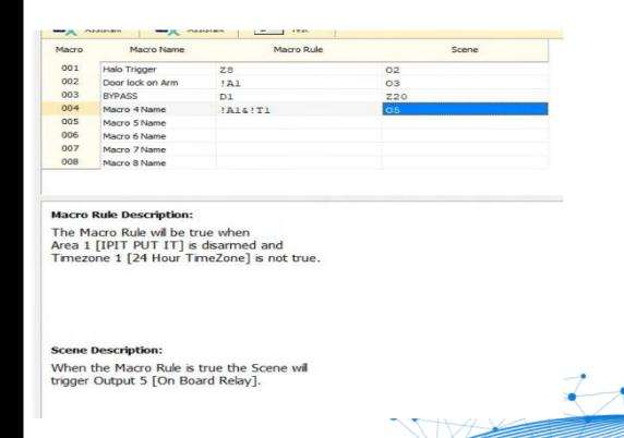
You can test the Macro Rule Test by clicking the triggers on the left changing the states of the triggers to make sure programming is correct
